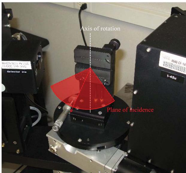
Fig. 2. (Color online) Details of the IR-VASE system with axis of rotation (in white) and plane of incidence with surface normal (in red) indicated.
